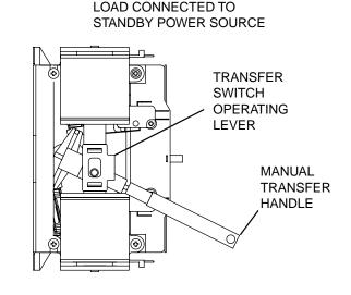
Figure 1. Manual Operation "V-Type" Switch
